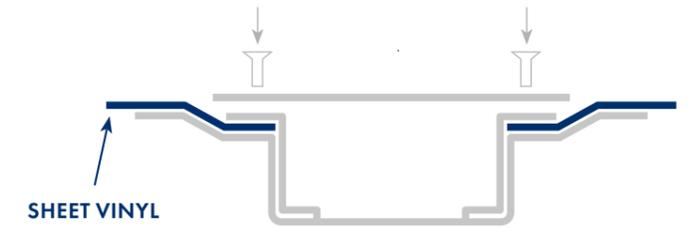
Only drains that have been specifically designed for use with sheet vinyl flooring should be considered in wet areas. These drains have clamping rings which prevent the ingress of water to provide a watertight finish.
